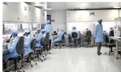
Clean Rooms - Class 10,000
