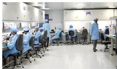
CLEAN ROOMS -CLASS 10,000
