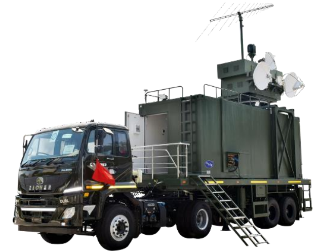
T&E Facility for Radar EW Systems
