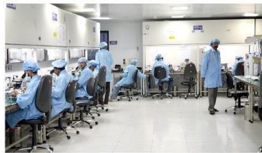
CLEAN ROOMS -CLASS 10,000
