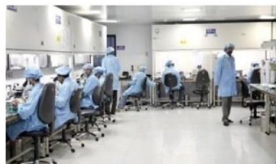
Clean Rooms - Class 10,000
